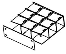
5. GLUE SIDE PANELS INTO POSITION. GLUE AND INSERT FEET.
