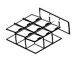
4. CONTINUE INSERTING SHELFS AND PLACING LOCKER DOORS FOR 2ND AND 3RD ROWS. GLUE BASE IN POSITION.
