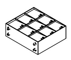
6. GLUE AND INSERT LOCKING CLIPS IN ALL LOCKER VOIDS. GLUE AND INSERT STOPPERS IN END COLUMN VOIDS.
