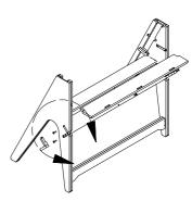
6. ASSEMBLE AND INSERT BACK PLATE
