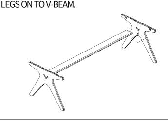
4. FLIP THE ASSEMBLY, PLACE CENTER BEAM AND BOLT IN PLACE.
