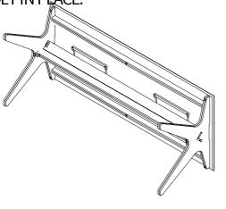
5. FLIP ASSEMBLY AGAIN AND DROP REMAINING BEAMS IN PLACE.
