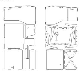
3. SAND AND OIL ALL REMAINING PARTS. INSERT NUTS IN BASE BOTTOM, SCREW BASE TO LEGS USING BOLTS
